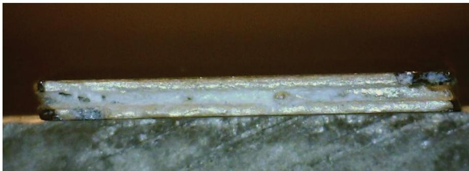
Figure 15: The TIM material inside a silicon diode.
