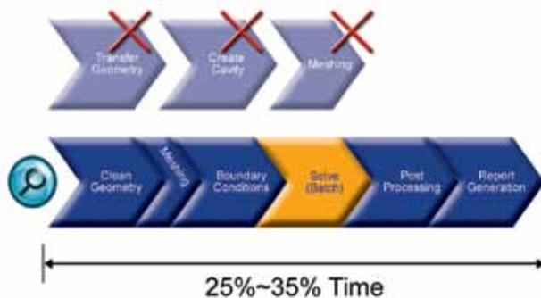
By comparison, Concurrent CFD works differently. The geometry used for the analysis is native to the CAD system. This means that geometry does not need to be transferred because the designer never has to leave the CAD system.
