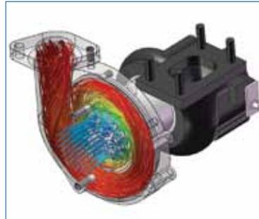
*FloEFD can show the visual results of 'Flow Field' analysis in several formats; shown here as stream lines that can be tracked from point of origin to point of exit*
