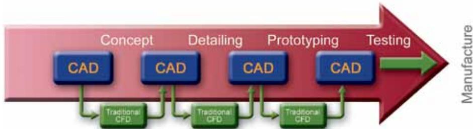
Upfront CFD attempts to improve this situation by streamlining the interface between the CAD and the CFD tool. Although this results in a much cleaner import of the geometry, the analysis is still performed outside of the CAD system. This frequent transfer from the CAD and CFD software can result in a degradation of your information.
