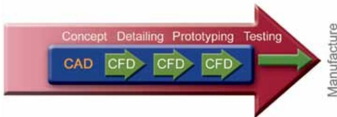
Concurrent CFD operates very differently. It is MCAD-embedded CFD so the work is done within the MCAD environment. Embedding CFD inside an MCAD tool is hard to accomplish, but delivers very significant benefits. Design changes necessary to achieve the desired product performance are made directly on the CAD model, so the design is always up-to-date with the analysis.
