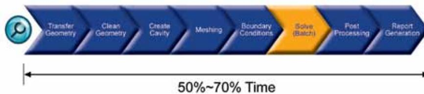
By looking at the CFD process in more detail, a number of steps are revealed. Within both conventional and upfront CFD it is necessary to transfer geometry from the CAD system and clean it before it is suitable for analysis. This process has to be repeated as design changes are made in the analysis suite and taken back into the CAD system to keep the two synchronized.
