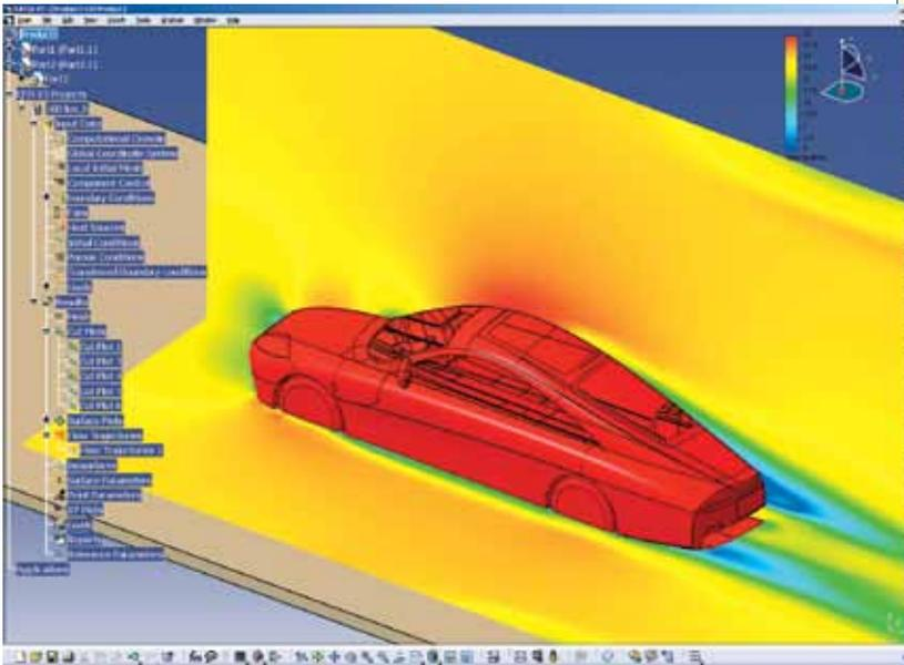
FloEFD for CATIA V5 is a fully embedded Concurrent Computational Fluid Dynamics (CFD) tool for CATIA V5. It enables you to study and optimize complex fluid flow and heat transfer effects on your designs directly inside CATIA V5 and faster than with any other CFD software.
