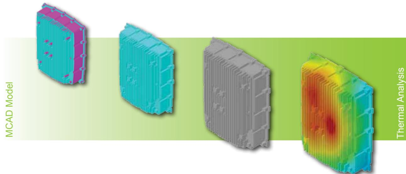
“ We use FloMCAD Bridge to simplify our original mechanical CAD files and quickly create computational models for the simulations. The way FloTHERM represents electronic components is a key advantage, enabling us either to use simple thermal data from component datasheets or switch to detailed 3D models for critical components when necessary. ”
