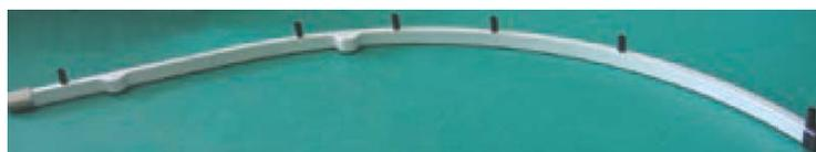
Part of microphone array with 6 channels, Lemo Connector on the end
