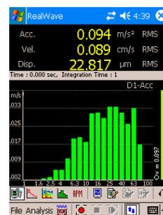
FFT based Octave Analysis and 3 mode of Vibration Measurement
