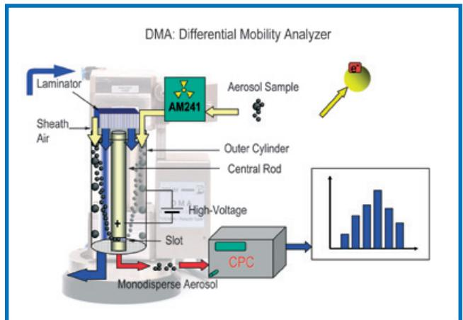
The DMA can also be used to generate monodisperse aerosols if operated at a fixed voltage.
