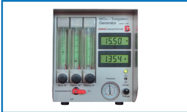
An indirectly heated Tungsten wire emits a large amount of oxide particles. Size and concentration can be set by adjusting the three air flows.
